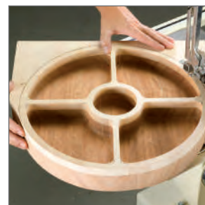
Bandsaw the exterior to final shape.
