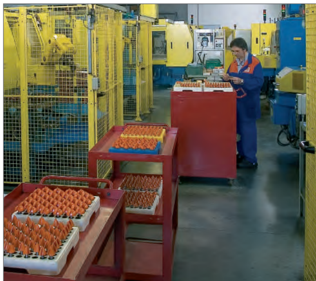
Loading the automated multi-axis CNC sharpening machines.
