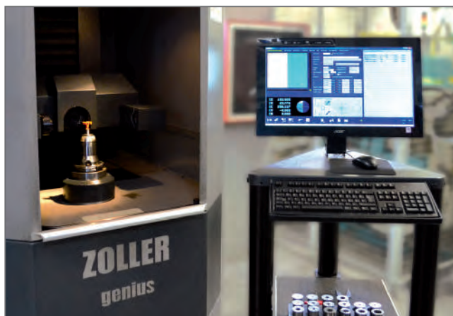
CMT's fully automatic measuring system.
