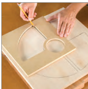
Trace the templates onto the bowl blank.
