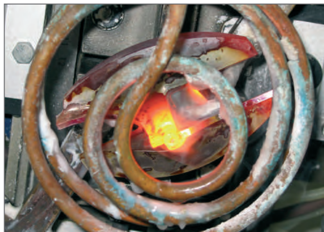
680°C in seconds - and the brazing is complete.
